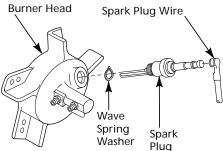
Figure 13 - Spark Plug Removal
